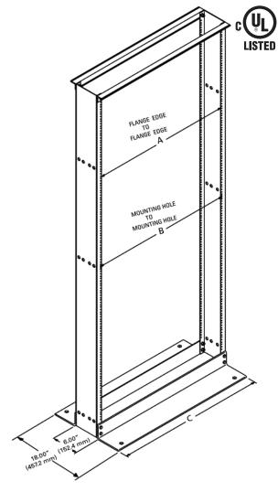
P/N 66363 (35" W) Shown: The 6"D (150 mm) Standard Rack is the high-capacity frame that is designed for use with cabling sections and is the basic frame around which the XLBET/MDF frames are developed.
