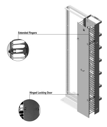
The CCS - EFX Combination Cabling Section - Extended Finger Xtra Capacity is a double-sided vertical cable management trough designed for use with CPI's Universal and Standard Racks to manage cable at the cross-connect, especially when using angled-face copper patch panels.
