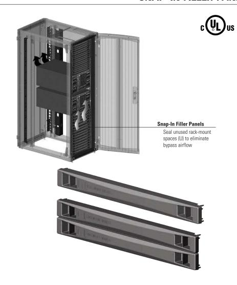
The Snap-In Filler Panels are solid panels used to fill open rack-mount spaces (U) in cabinets that store rack-mount computer servers and data storage equipment. Designed to occupy the entire rack-mount space (U) height eliminating leakage between stacked panels.
