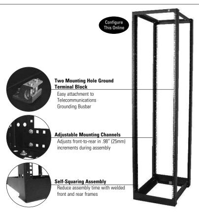
The Adjustable ServerRack and the Adjustable QuadraRack® provide a sturdy, cost-effective solution for supporting rack-mount network, computer server and data storage equipment in data centers, computer equipment rooms and other IT facilities. Both racks offer the strength and stability of an enclosure in an open four-post frame that provides easy access to equipment and cabling.
