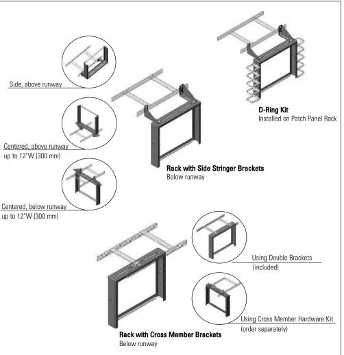
Cable Runway Patch Panel Rack is a miniature two-post rack that can be attached to CPI Cable Runway. Cable Runway Patch Panel Rack saves rack-mount space in a rack or cabinet that stores computer and data storage equipment by placing patch panels or interconnect equipment above the rack or cabinet. Use Cable Runway Patch Panel Rack to create a zone network in the data center.
