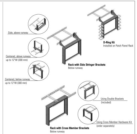
Cable Runway Patch Panel Rack is a miniature two-post rack that can be attached to CPI Cable Runway. Cable Runway Patch Panel Rack saves rack-mount space in a rack or cabinet that stores computer and data storage equipment by placing patch panels or interconnect equipment above the rack or cabinet. Use Cable Runway Patch Panel Rack to create a zone network in the data center.
