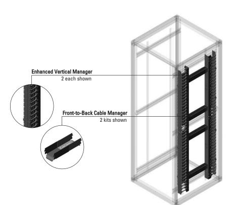
Enhanced Vertical and Front-to-Back Managers are accessories for the CPI M-Series MegaFrame<sup>®</sup> Cabinet System. MegaFrame Cabinet features integrated cable management space along both sides of the cabinet frame. Cable managers used within this space can be adjusted in depth (front-to-rear) to align cables with equipment.
