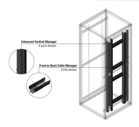
Enhanced Vertical and Front-to-Back Managers are accessories for the CPI M-Series MegaFrame® Cabinet System. MegaFrame Cabinet features integrated cable management space along both sides of the cabinet frame. Cable managers used within this space can be adjusted in depth (front-to-rear) to align cables with equipment.
