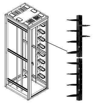
Rings on the MegaFrame Vertical Cable Manager can be oriented in parallel or perpendicular to the cabinet's mounting rails. Use the Manager as show near the rear of the cabinet to create two pathways for cabling with one manager.
