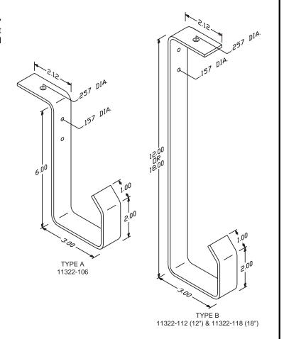
Part Number Dim A Description Type 11322-106 6" Α 6" J-Hook Bracket 11322-112 12" В 12" J-Hook Bracket 18" В 11322-118 18" J-Hook Bracket
