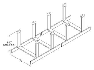
Note: When using P/N 10693 select a radius drop that is less than 7.5"W (191 mm) such as P/N 12101-X03.
