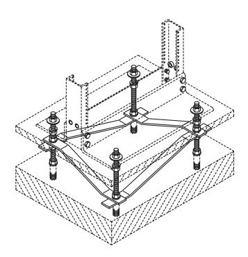
Raised Floor Rack Support includes all the hardware you need to install a CPI Standard, Universal or 6" Deep Standard Rack over a raised floor.
