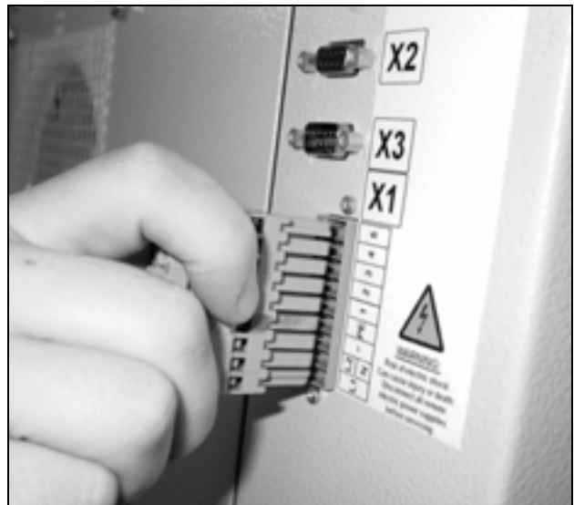
Fig. 28: Disconnect the mains plug
