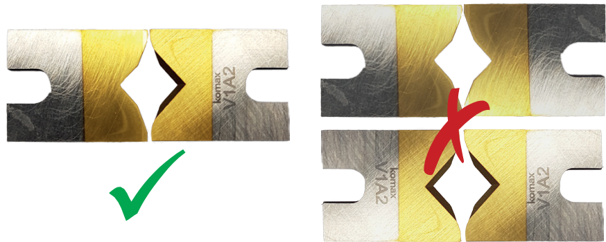
Fig. 14: Aligning the blades
