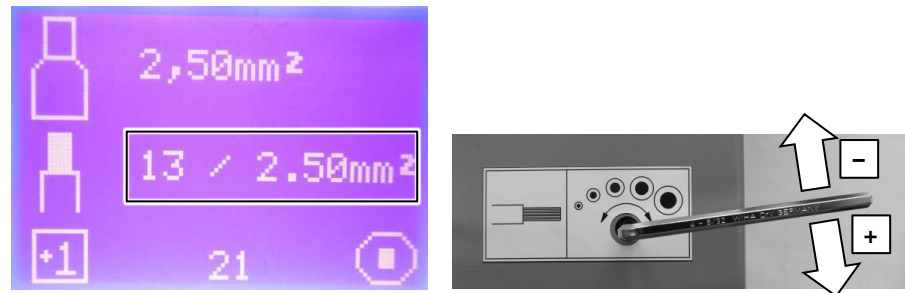
Fig. 9: Insulation stripping stage setting
