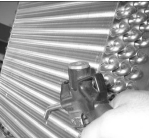
Fig. 30: Clean the heat exchanger coil and compressor chamber using compressed air
