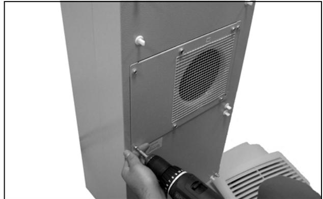
Fig. 63: Undo the four screws for the external circuit fan
