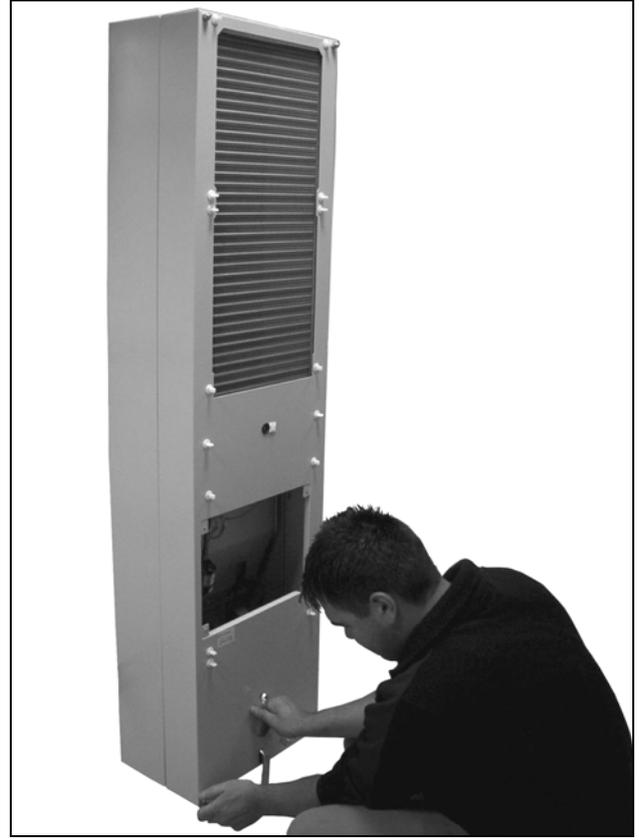
Fig. 70: Undo the four screws for the cover
