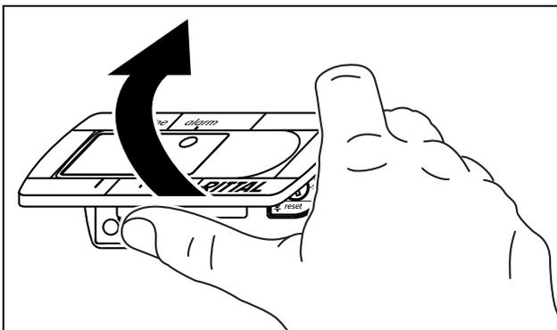
Fig. 29: Releasing the Basic controller trim panel
