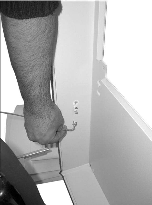
Fig. 73: Disconnect the earthing cable (2)
