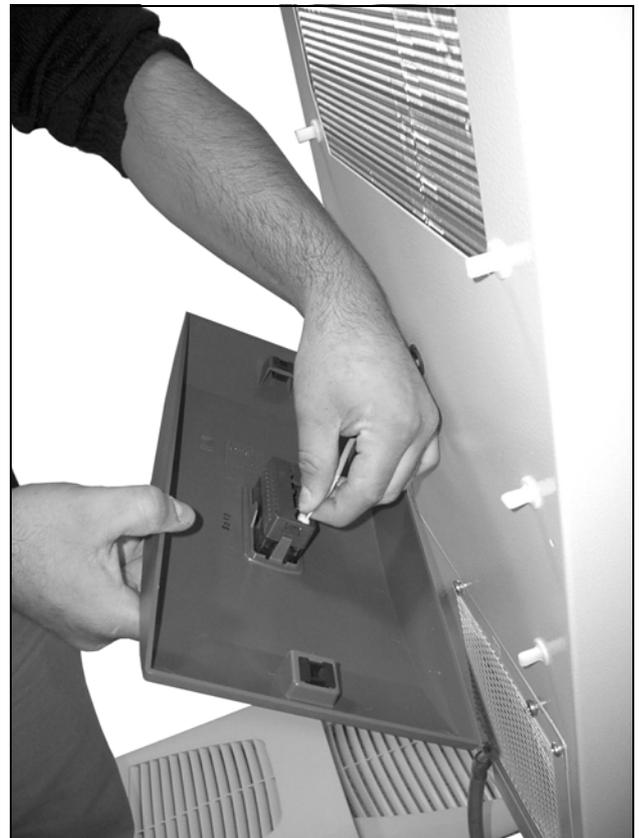
Fig. 38: Disconnect the connector from the display (1)
