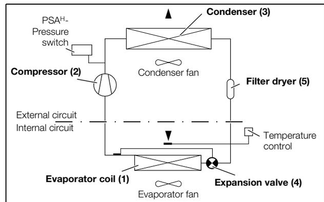
Fig. 3: Cooling circuit
