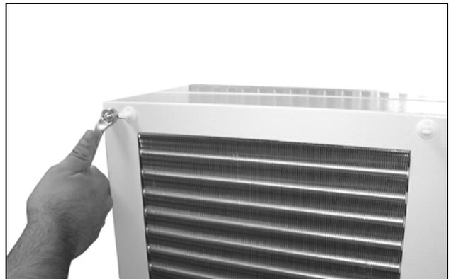
Fig. 44: Remove the cover (undo the four nuts)
