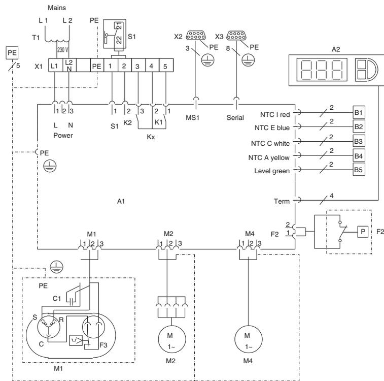
Fig. 113: Electrical wiring plan no. 3
