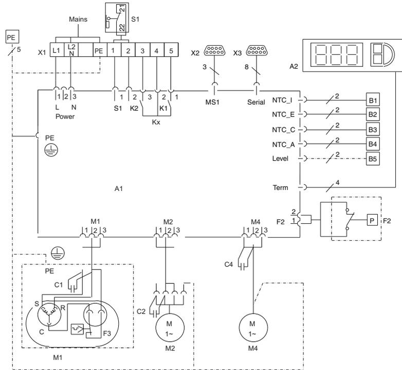
Fig. 112: Electrical wiring plan no. 2
