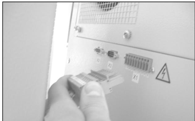
Fig. 34: Disconnect the mains plug
