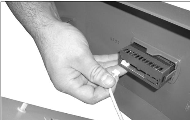
Fig. 60: Disconnect the display cable
