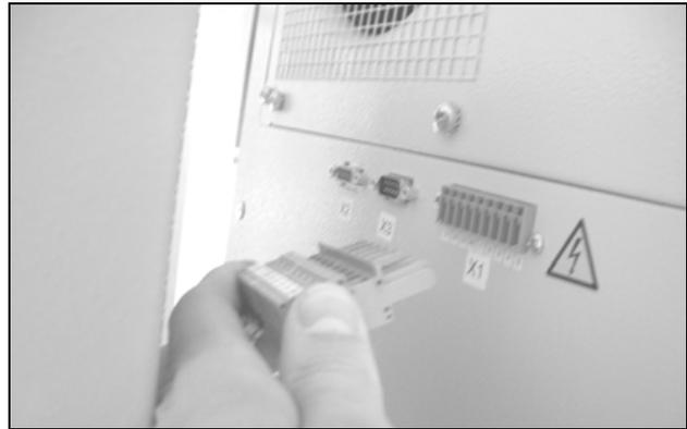
Fig. 53: Disconnect the mains plug
