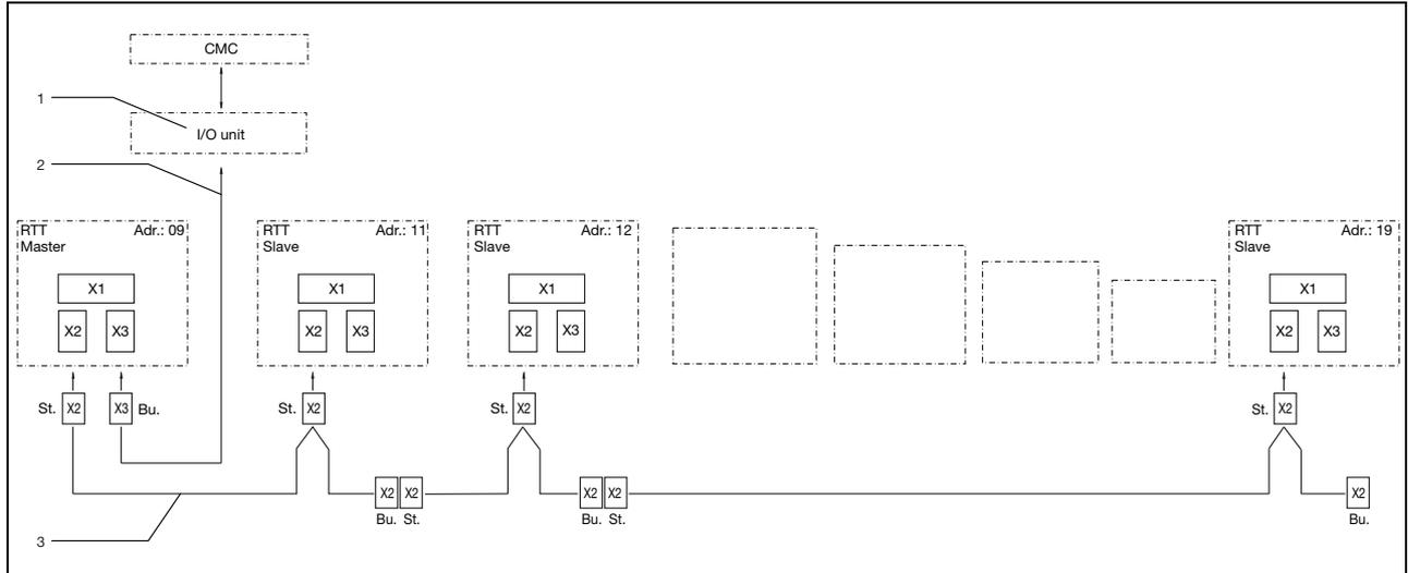
Fig. 21: Connection example: Master-slave operation
