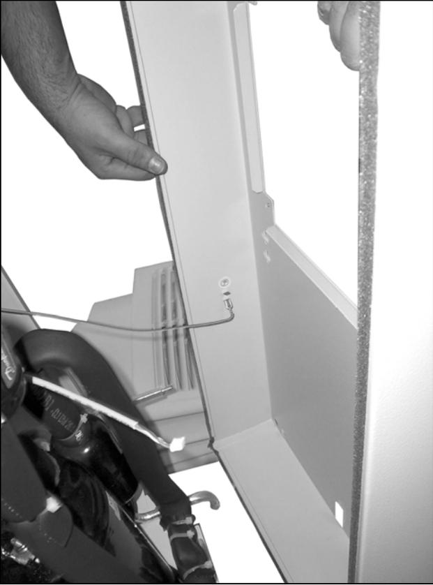
Fig. 72: Disconnect the earthing cable (1)
