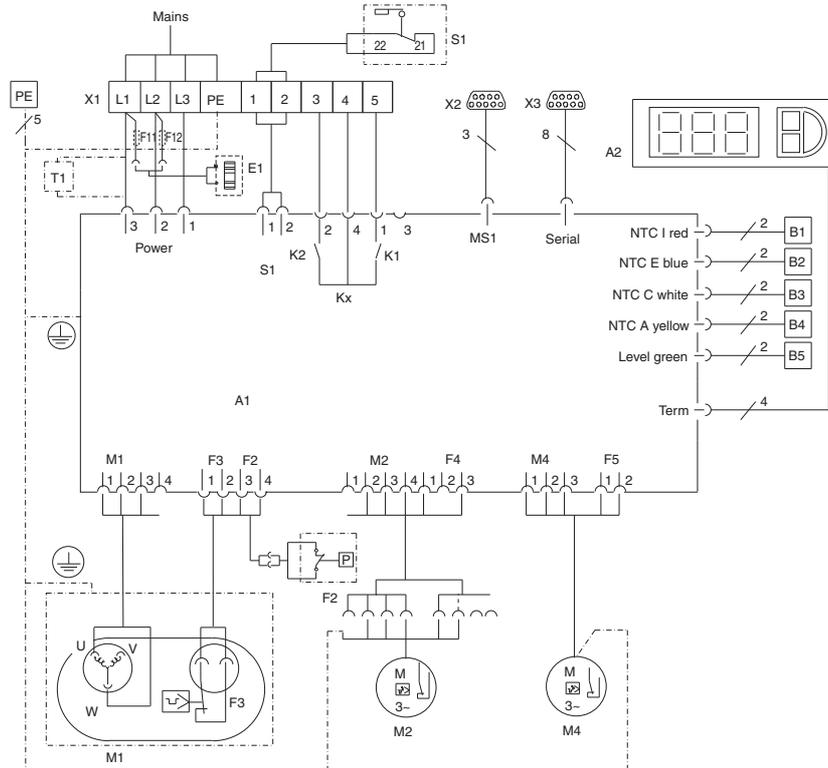
Fig. 116: Electrical wiring plan no. 6
