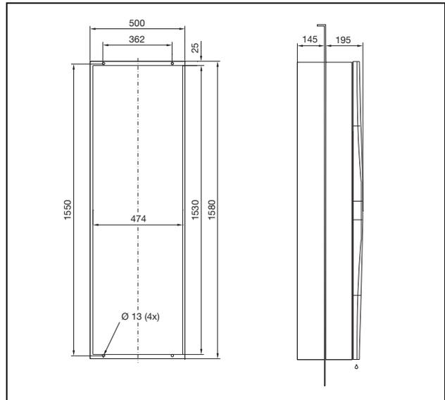
Fig. 104: 3332.xxx partial internal mounting
