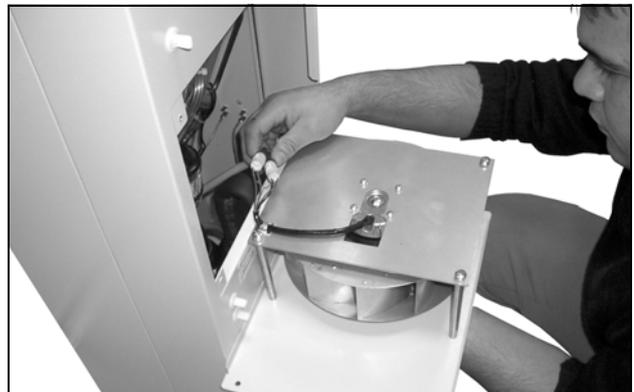
Fig. 65: Disconnect the fan connectors (1)
