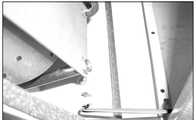
Fig. 49: Release the earthing cable between the cover and the chassis (1)
