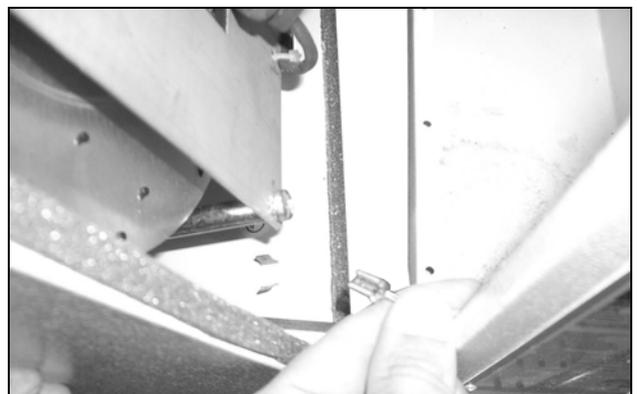
Fig. 50: Release the earthing cable between the cover and the chassis (2)
