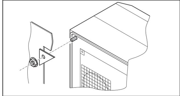
Fig. 9: Securing the cooling unit (3302.1xx only "external mounting")
