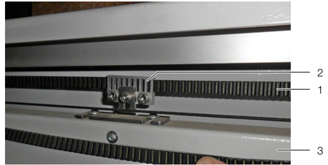
Fig. 36: Fasten the toothed belt to the left-hand door
