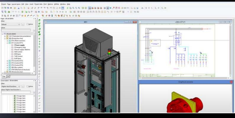
With RiCAD 3D, you have validated CAD data at your fingertips for professional design planning. Make use of the original CAD data of the Rittal components – irrespective of your particular CAD system. Even more efficient planning is possible with EPLAN Pro Panel, the leading software solution for project planning and 3D engineering.
