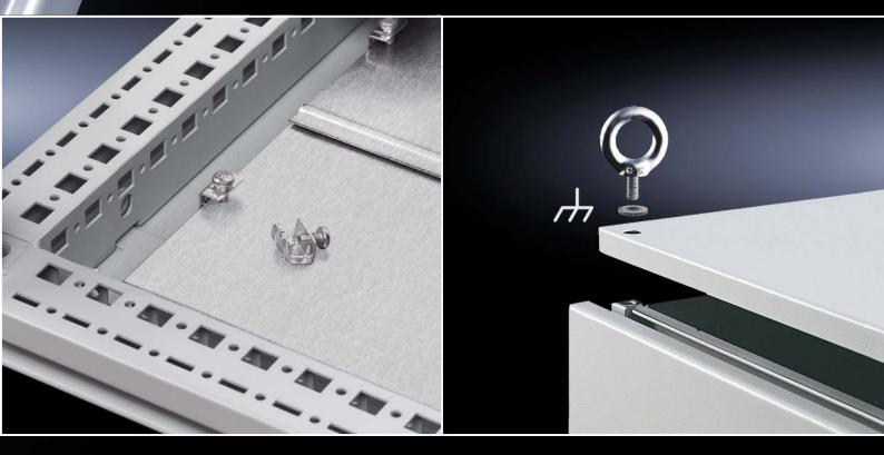
Potential equalisation for the gland plates, side panels, rear panel and roof is achieved automatically when the enclosure is assembled. That guarantees a conductive contact between the frame and all panel parts. Where there are no electrical devices mounted on the panel parts, it is possible to forego earth straps.
