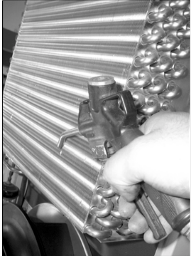
Fig. 82: Clean out the heat exchanger coil and compressor chamber using compressed air (2)
