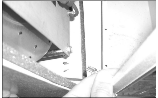
Fig. 57: Loosen the earthing cable between the cover and the chassis (2)
