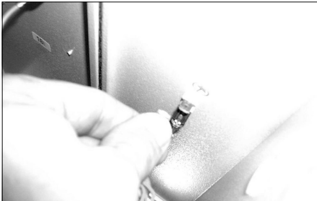
Fig. 76: Disconnect the fan earthing cable (2)
