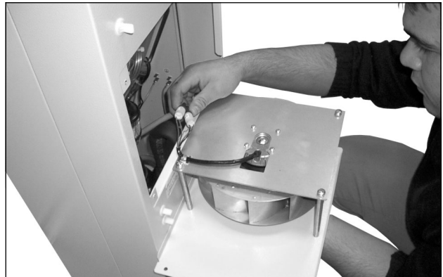
Fig. 72: Disconnect the fan connectors (1)
