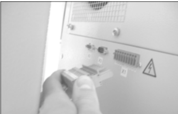
Fig. 60: Disconnect the power cord
