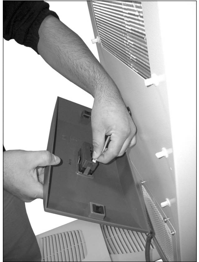
Fig. 45: Disconnect the connector from the display (1)
