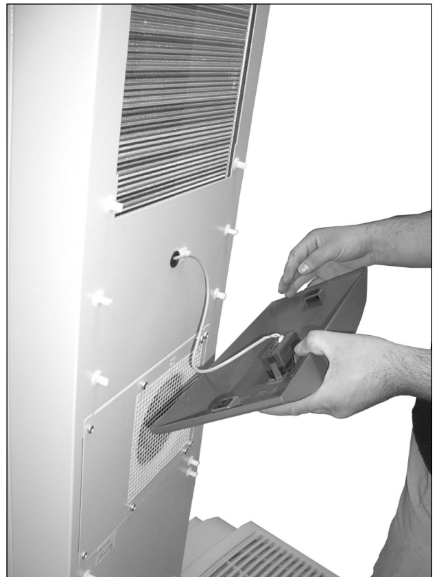
Fig. 66: Remove the infill panel
